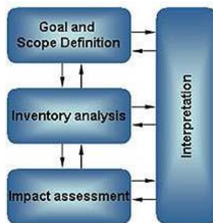
Figure 2. Four phases in an LCA study, beginning with goal and scope definition, followed by inventory analysis, impact assessment and interpretation. 31
